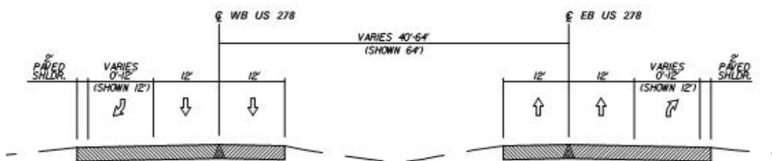
**Figure 3-1. Typical Section of Existing US 278 Roadway**
