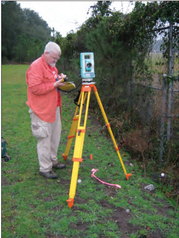
Figure 3.4 Mapping features at 38BU2301 using a laser theodolite.
