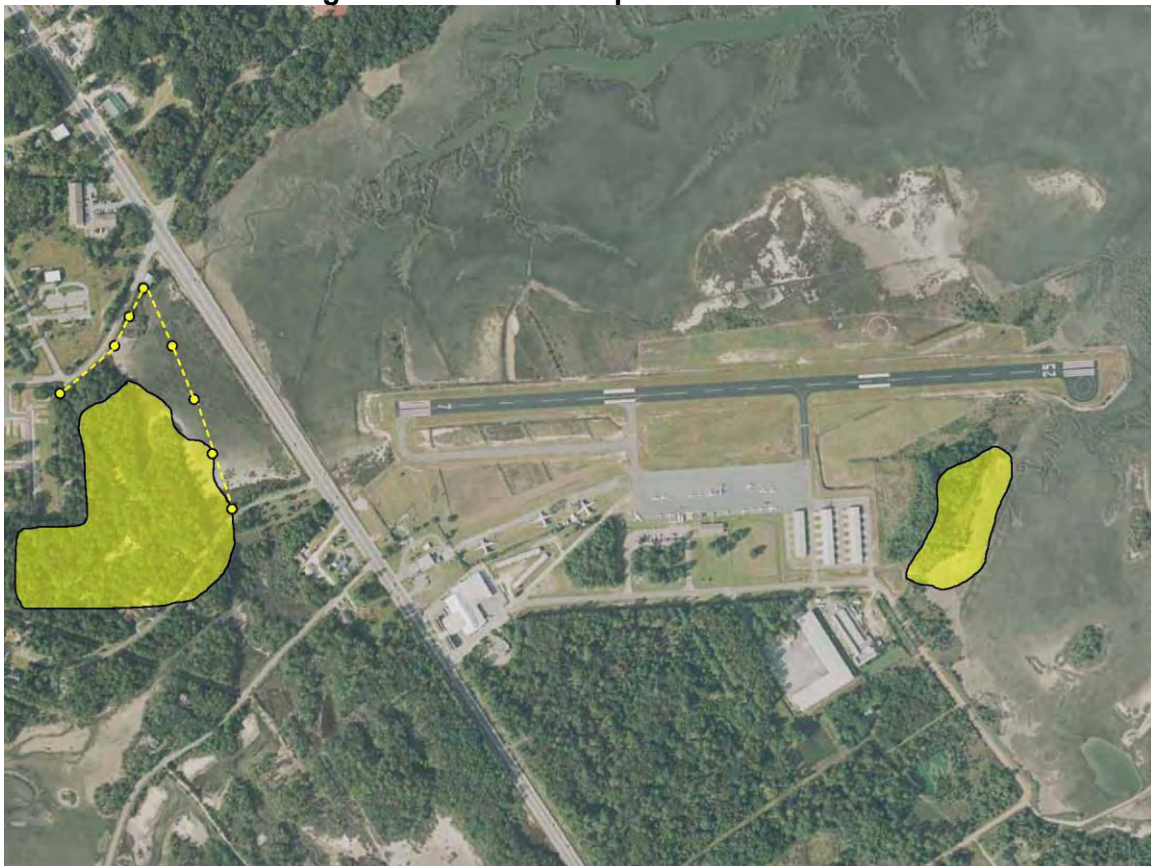
Figure 1-6: Current Airspace Obstructions
